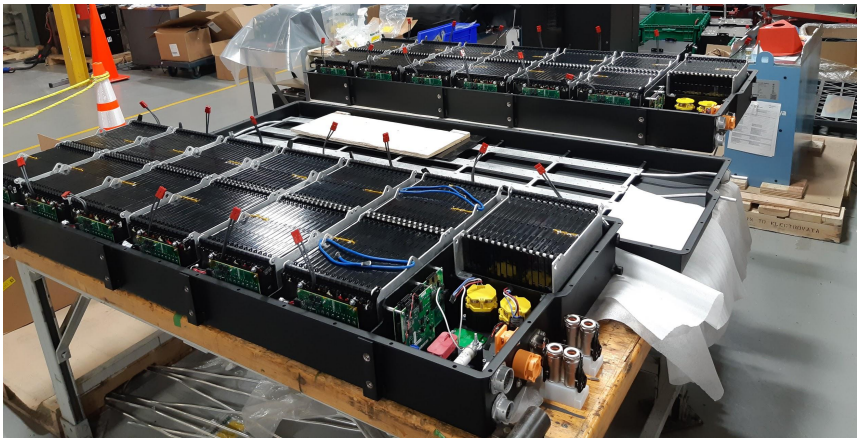
Electrovaya 670V battery packs under assembly
